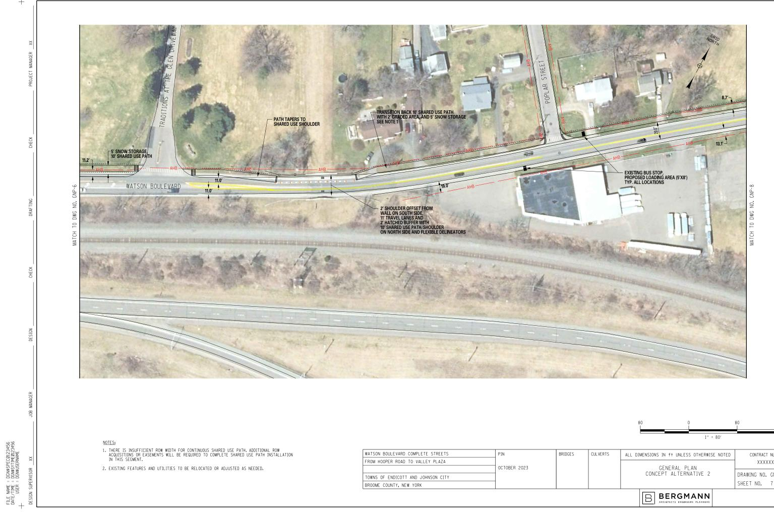
THERE IS INSUFFICIENT ROW WIDTH FOR CONTINUOUS SHARED USE PATH. ADDITIONAL ROW ACQUISITIONS OR EASEMENTS WILL BE REQUIRED TO COMPLETE SHARED USE PATH INSTALLATION IN THIS SEGMENT.
