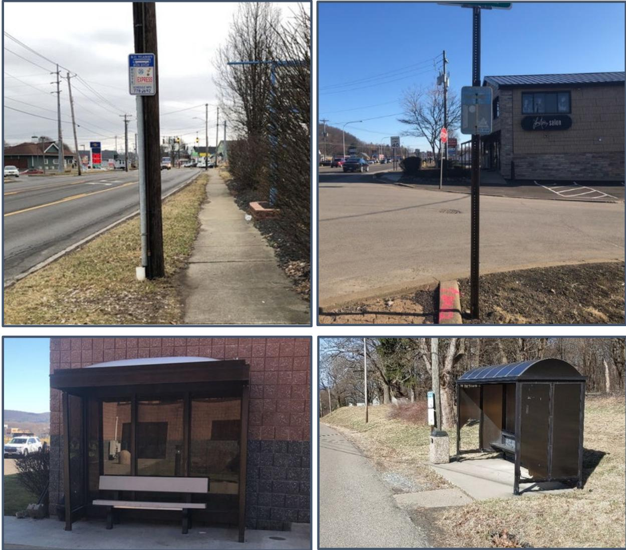
*Figure 3 - Examples of Typical Conditions of Bus Stop Signs Classified 'Good' (top-left) and 'Poor' or 'Damaged' (Top-Right), and Bus Shelters Classified as 'Good' (bottom-left) and 'Poor' (bottom-right).*
